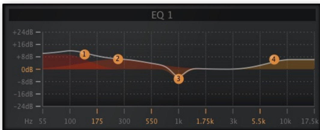
Equalizer module, bass+treble boost, dip around 1.5 kHz
