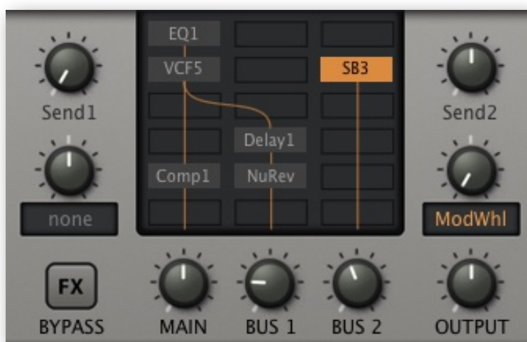
FX Grid with example routing
